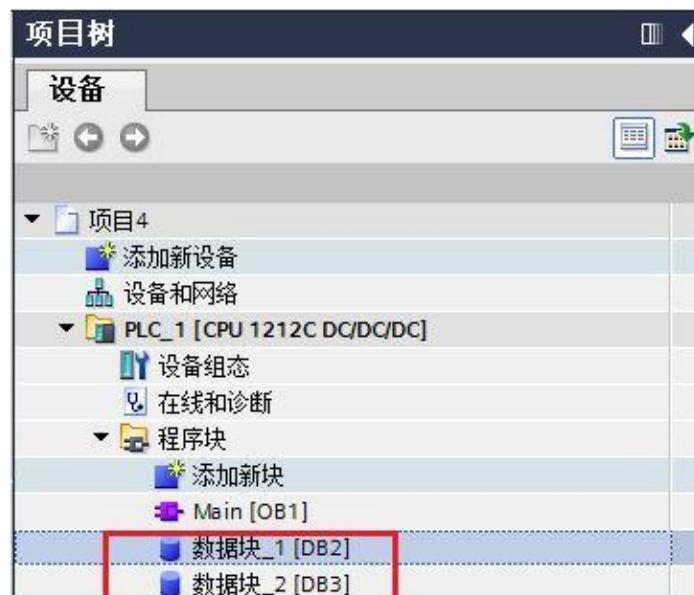
The second step is to establish a Word array data type to store data during communication, as shown in the figure.
