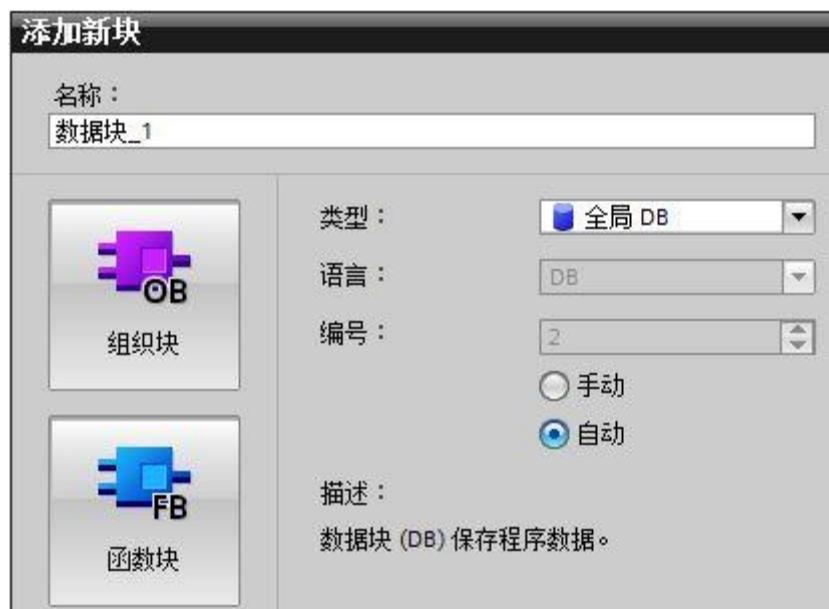
In the second step, double-click to open DB2, define the variable name as "aa", and the data type as "TCON\_IP\_v4" (TCON\_IP\_v4 can be copied to this dialog box), and then click the "Enter" button. The data type structure is created:
