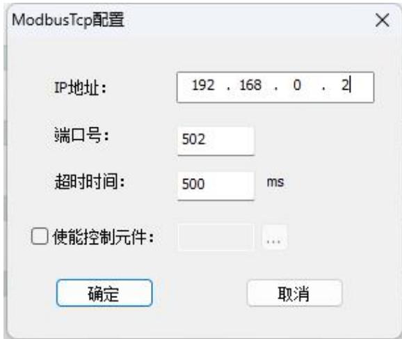
After clicking OK, a Modbus TCP connection device will be added:
