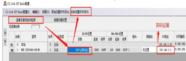
6.To refresh the target, select the specified device-software name M-assign the device address-application, and the configuration is completed!
